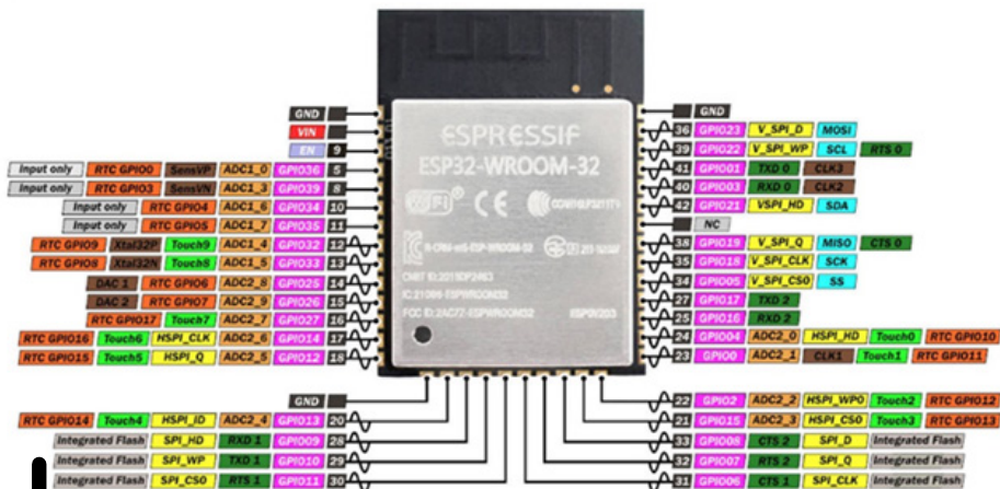
Figura 4. Pinout del ESP32 Wroom-32.
